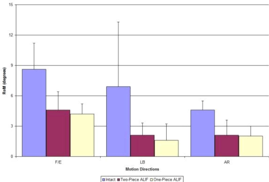
[Fig. 1. RoM for Intact and 360 ALIF Devices]
